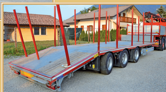
BP28WX - Particolare del 3° asse sterzante e sbalzo posteriore inclinabile Detail showing steering 3rd axle and rear end tilting bed Detail der 3. lenkenden Achse und hintere neigbare Auskrugung
