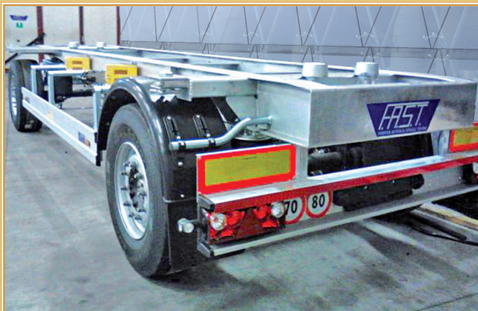
BP18CM - Rimorchio FAST per trasporto casse mobili unificate FAST trailer for transporting standard freight containers FAST Anhänger zum Transport von Standardcontainern
