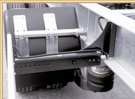
Sollevatore 1° asse automatico Automatic axle lift for the 1st axle Automatische Hebevorrichtung f. 1. Achse
