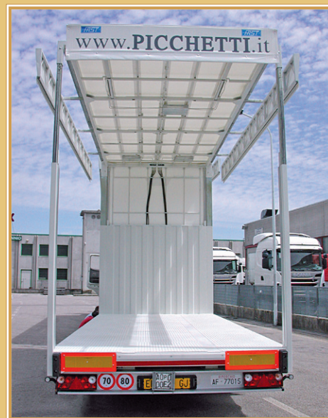
Tetto idraulico sollevabile Hydraulic lift-up roof hydraulisch anhebbares Dach
