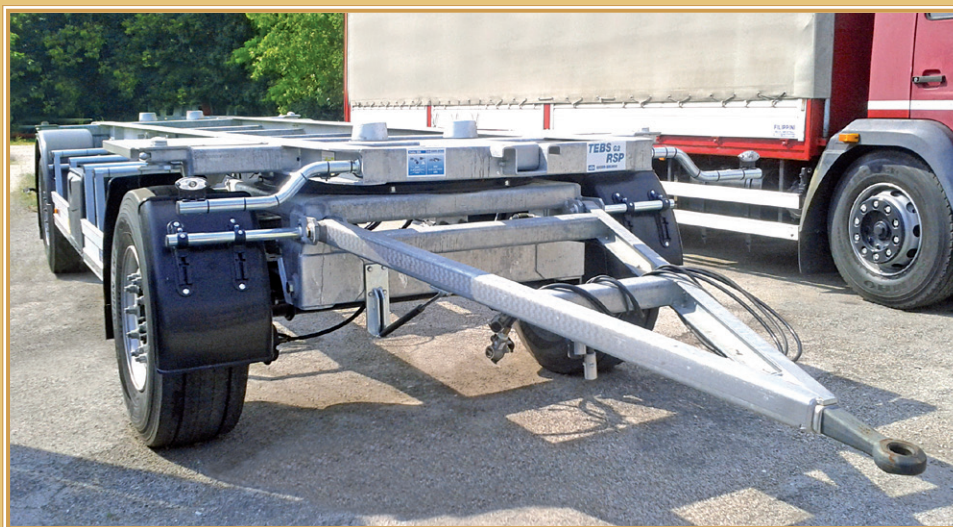
BP18CM - Rimorchio FAST per trasporto casse mobili unificate FAST trailer for transporting standard freight containers FAST Anhänger zum Transport von Standardcontainern
