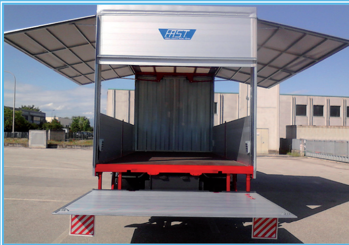
12- Sponda a battuta posteriore: particolare Pedana aperta Rear liftgate: view of the opened platform Ladebordwand: Detail Trittläche offen
