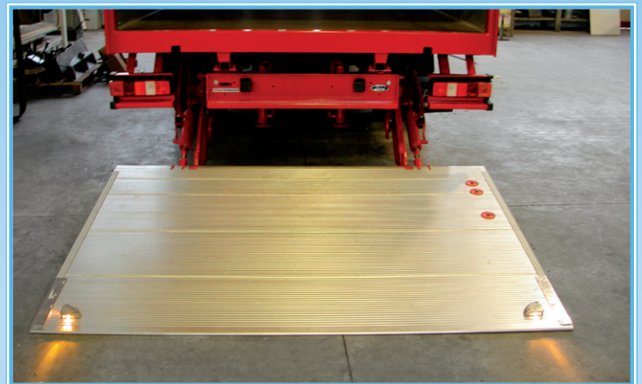
18- Pedana ripieghevole: particolare luci a led zona punta Folding platform: detail of extremity lights and LEDs Faltbare Trittläche: Detail Led Beleuchtung im Randbereich
