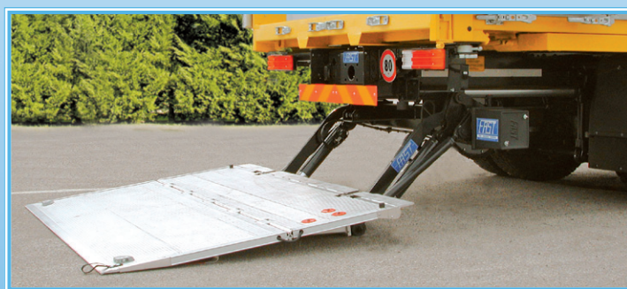
7- Pedana a semplice ripiegatura: raccordo automatico a terra Single folding platform: automatic contact with the ground Einfach faltbare Trittläche: automatischer Anschluss an den Boden
